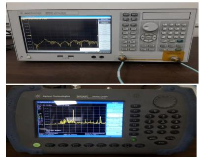
**High-performance Spectrum Analyzer:** 3 Hz to 8.4 GHz , Preamplifier up to 8.4 GHz, External Mixing Option available.
